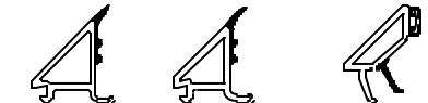
28mm Ext. Bead P50033 28mm Ext. Bead P10134 28mm Single leg bead P50129
